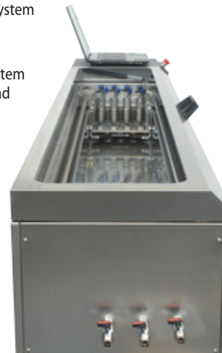
Detail of water bath. Easy and free access to the large testing space, common to all versions
