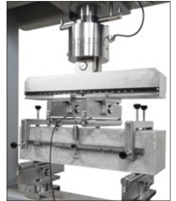
Beam deflection test on FRC concrete to ASTM C1609
