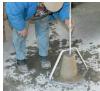
54-C0149/B, 54-C0150/C during use. The handle raises up over specimen and slump is measured using the tamping rod which is engraved with 1 cm graduations.
