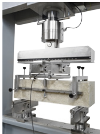
Beam deflection test to ASTM C1609 including two high precision LVDT displacement transducers and auxiliary frame
