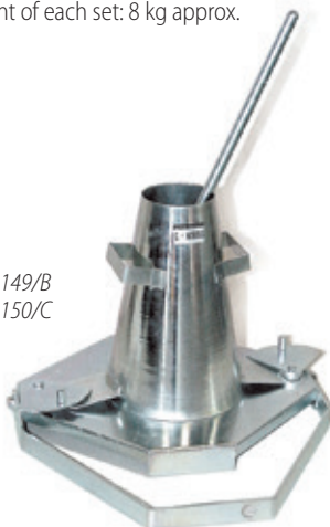
54-C0149/B, 54-C0150/C during use. The handle raises up over specimen and slump is measured using the tamping rod which is engraved with 1 cm graduations.
