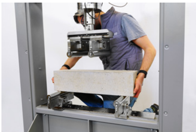
SIMPLEX models feature direct operator's access to the frame allowing easy frontal loading and positioning of specimens or heavy test accessories
