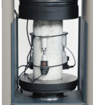
Three compressometer-extensometers 55-C0222/G fitted to a cylindrical specimen during compression stage.
