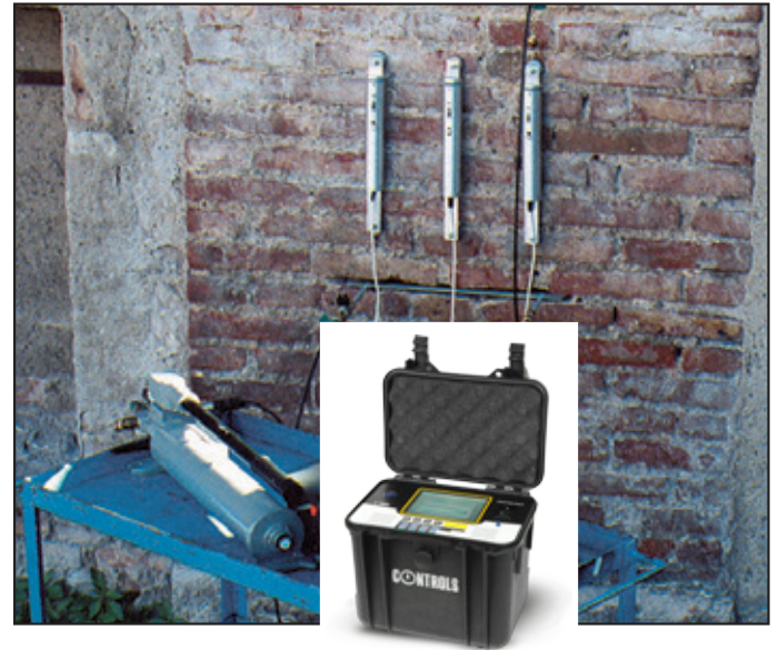
Typical application with digital configuration composed with 3 electronic tubular transducers 58-D0585, pump assembly 58-D0568 fitted with pressure transducer 82-P0050, suitable cable P0349/ELT and DATALOG 8 82-P9008 for complete data acquisition.
