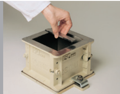
Verification of a cube mould with Go/No go gauges
