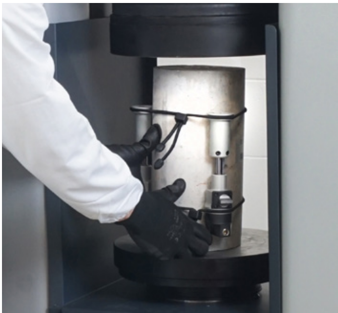
Elastic modulus determination with Automax Pro-M 3000kN EN compression machine, upgraded with 50-FW/EM.
