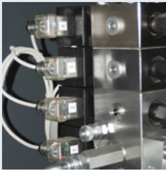
AUTOMAX fitted with 50-C10D/3F and 50-C20E/4F valves for connection and control of a third and fourth frame
