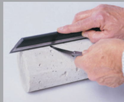
Straightness verification using straight edge 82-C0108/1 and set of feeler strips 82-C0110/1
