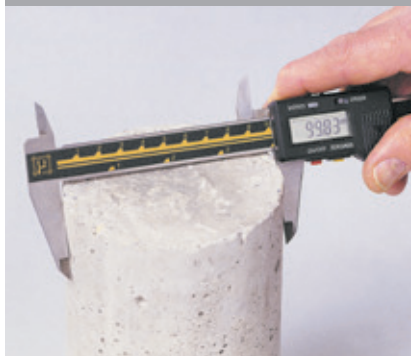
Verification of diameter using Digital Vernier caliper 82-C0109/1
