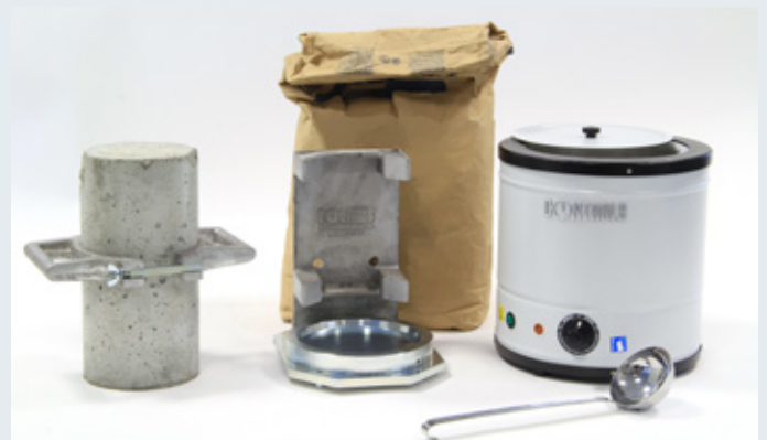
Sulphur capping equipment
