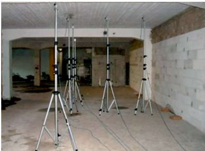
Digital instrumentation for deflection measurement of structures, complete system with 3 additional measurement elements
