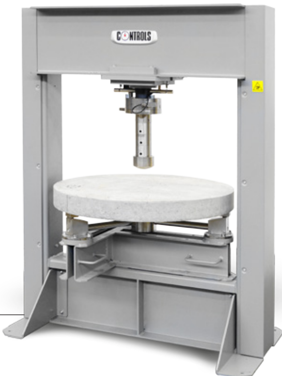
50-C1711/FR with C1700/7 and C1500/8 for round slab testing to ASTM C1550
