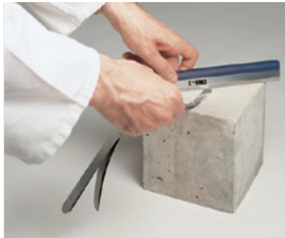
Flatness verification using straight edge 82-C0108/1 and set of feeler strips 82-C0110/1
