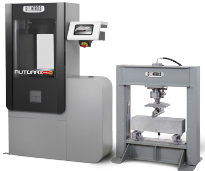
CMOD test performed on the 200 kN flexure frame C1511/FR controlled by the AUTOMAX PRO-M system upgraded with 50-FW/DC.
