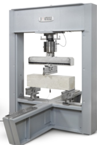
50-C1701/FR with bearers 50-C1700/1 during CMOD test: FRC beam is kept parallel to the frame for maximum stiffness
