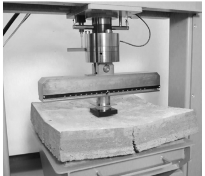
Testing FRC square slab to EN 14488-5 on 350 kN DUPLEX flexure frame 50-C1701/FR
