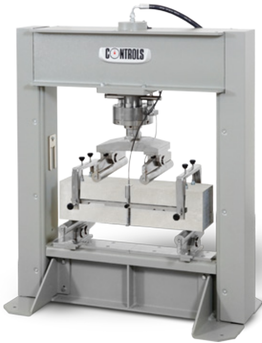
50-C1511/FR with bearers 50-C1500/1, auxiliary frame 50-C1500/5 and two LVDT transducers 82-P0331/C for flexural test on FRC beam to ASTM C1609
