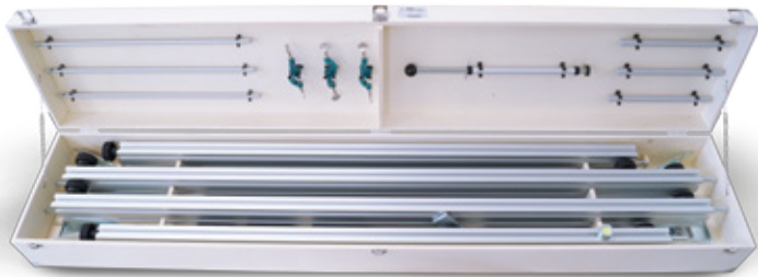
Complete measuring bar 5.5 meters long and adjustable supports for displacement devices housed inside the wooden carrying case
