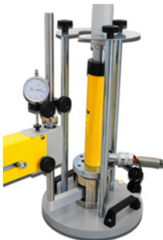
Detail of the hydraulic assembly of 35-T11D1: load plate diameter 300 mm; hydraulic cylinder with spherical seat and extension rods; telescopic arm; measuring tunnel; anti tilting 3-column jig and dial gauge
