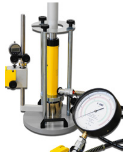
Detail of the hydraulic assembly of 35-T11D1: triple scale manometer and digital gauge 82-D1262/B
