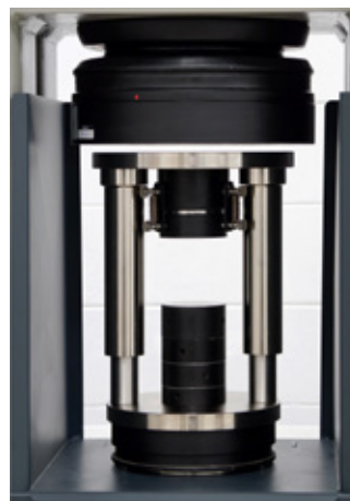
Compression device for rock specimens model 32-D9035 mounted inside a CONTROLS compression machine
