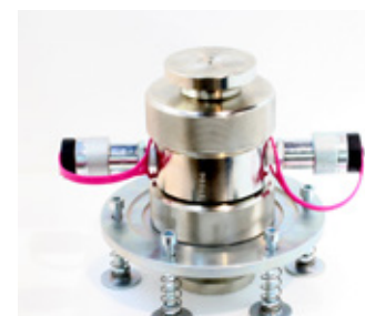
Hoek cell supported by holding device
