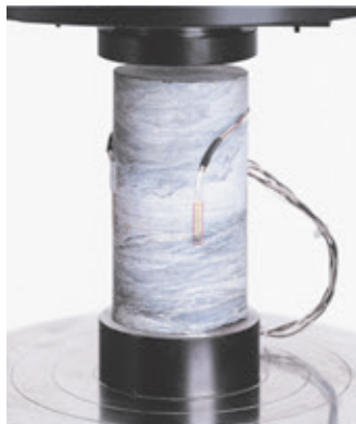
Rock sample fitted with 82-P0390 strain gauges
