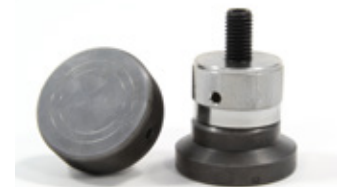
32-D0550/D5 Set of lower and upper platen 52 mm dia. with spherical seat model for compression tests
