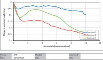
Example of a direct shear test processed with the 30-WF6008/T2 Geo-Analysis template (BS EN ISO standard): the top plot shows shear stress versus horizontal displacement; the bottom plot shows change in specimen height versus horizontal displacement
