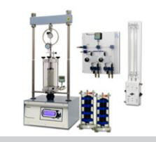
**Triaxial System with analog measurements** is the ideal basic solution to perform standard triaxial tests, such as effective and total stress, for laboratories that don't require digital measurement. All the data acquisition and test management are made in manual mode.
