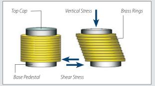
Schematic Stress condition of the sample in the cyclic simple shear
