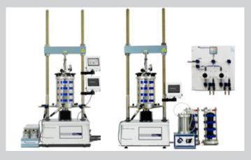
**Triaxial System with automatic built-in data acquisition** is the simplest compact solution for standard triaxial testing (effective and total stress). It can be equipped with standard air/water interface pressure system or with automatic pressure/volume controllers. No requirement for external data acquisition and/ or PC.
