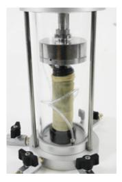
Detail of standard triaxial cell fitted with submersible load cell
