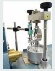
Detail of Shearmatic EmS fitted with Consolidation accessories and consolidation cell for automatic performance of the consolidation test
