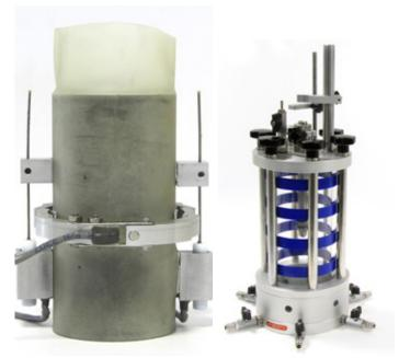
Transducers mounted on a sample
