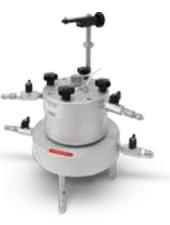
26-WF0346 Hydrocon SWCC consolidation cell for 100 mm diameter unsaturated samples.
