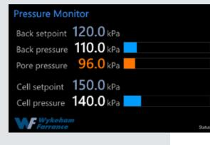
Cell, back and pore pressure monitoring via high resolution 7" color touchscreen display
