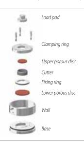
Exploded view of consolidation cell 26-WF0320
