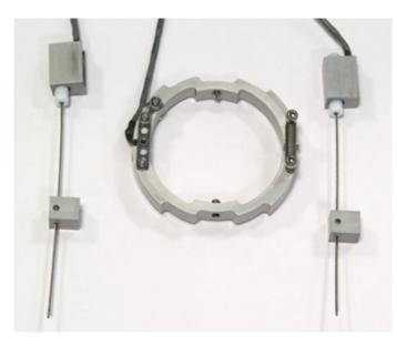
Local strain transducers are supplied in a kit which includes one radial and two axial transducers suitable for 38mm, 50mm,70mm, 100mm and 150mm specimen diameters. Mounting accessories such as radial belt, mounting brackets and jig are also included.
