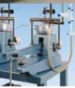
Three oedometers 26-WF0302, complete with cells, 30-WF6207 displacement electronic transducers connected to 30-WF6008 GEODATALOG, and 26-WF0312 consolidation bench.
