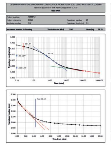
*Example of a consolidation test analysis with the 30-WF6008/T8 Geo-Analysis template (ASTM standard), t50 and T90 calculations*
