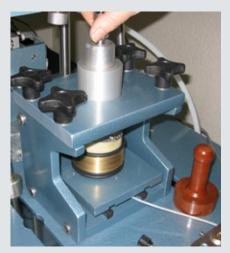
Sample Preparation using wooden dolly included the machine.
