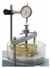
Detail of shar box case fitted in analog mode
