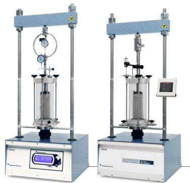
TRIAX fitted with standard triaxial cell, dial gauge and load rings; TRIAX with 4 built-in channels fitted with standard triaxial cell, external load cell and displacement transducer.
