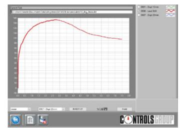
Real time raw testing data coming from 5 kN load during direct shear test
