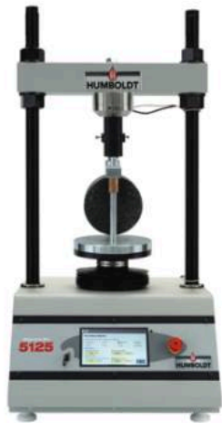
IDEAL-CT (TTI Method) ASTM D8225
