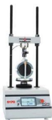
HM-5170A.3F showing Marshall setup
