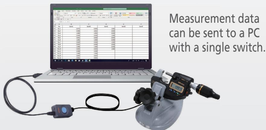
Measurement data can be sent to a PC with a single switch.
