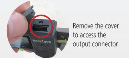
Remove the cover to access the output connector.
